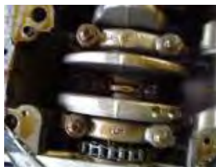
Fig 4: Bottom end of engine showing crank and rods with detail of crank and one rod
