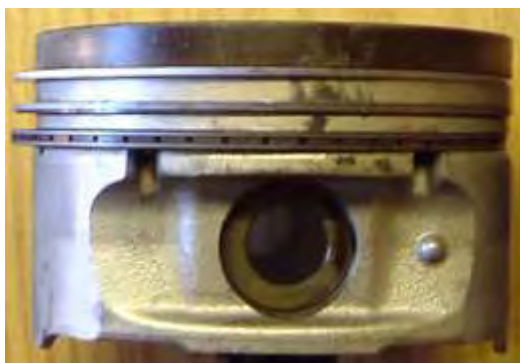
Fig 4: Prohibited domed piston. Remains prohibited even if machined flat.
