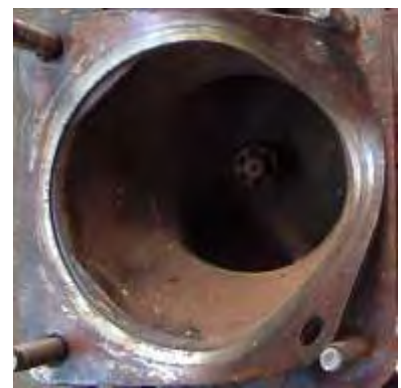
Fig 9: Prohibited Mk3 manifold
