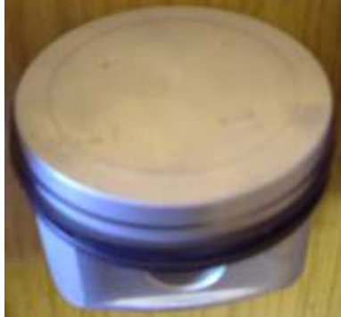
Fig 1: Permitted Mahle piston No:0400400. Weight 320g without gudgeon pin
