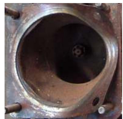
Fig 9: Prohibited Mk3 manifold
