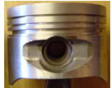
Fig 3: Permitted piston short skirt raised crown 0.75mm stamped 062 12
