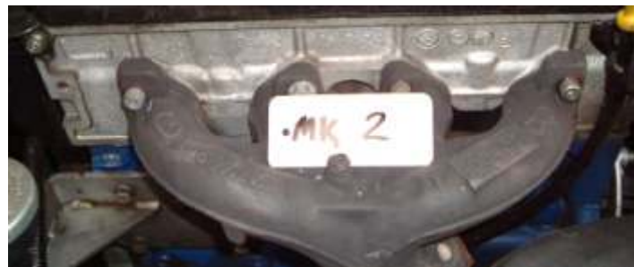
Fig 13: Permitted head Mk2
