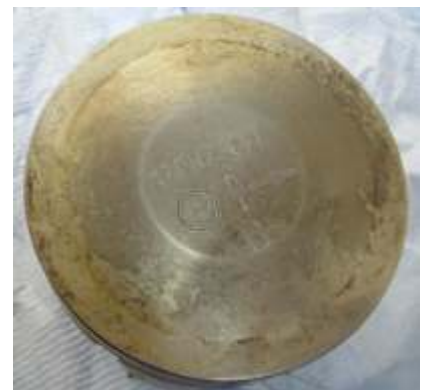
Fig 4: Prohibited domed piston. Remains prohibited even if machined flat.
