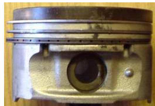
Fig 4: Prohibited domed piston. Remains prohibited even if machined flat.
