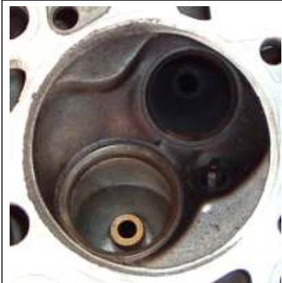
Fig 10: Permitted head Mk1
