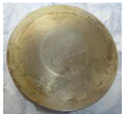
Fig 4: Prohibited domed piston. Remains prohibited even if machined flat.
