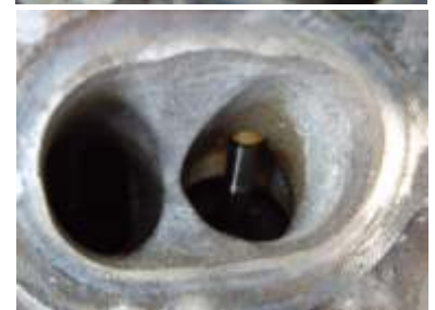
Fig 2: Inlet ports showing casting marks
