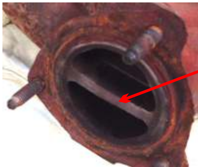
Fig 8: Permitted Mk1 & Mk2 exhaust manifold
