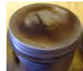
Fig 3: Long Skirt Protruding Crown - Prohibited
