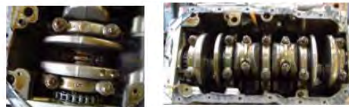
Fig 4: Bottom end of engine showing crank and rods with detail of crank and one rod
