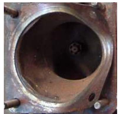
Fig 9: Prohibited Mk3 manifold
