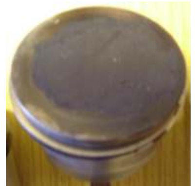
Fig 3: Permitted piston short skirt raised crown 0.75mm stamped 062 12
