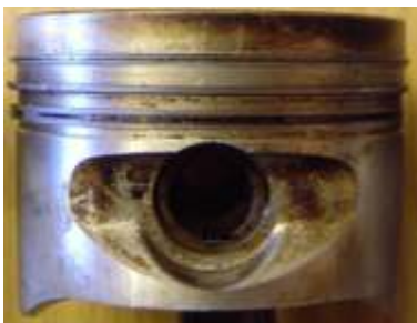
Fig 1: Permitted Mahle piston No:0400400. Weight 320g without gudgeon pin
