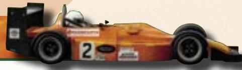
First introduced in 1949 by the 750 Motor Club, 750 Formula is the longest continually running race formula in the world. The regulations provide ample scope for the amateur to design and build their own car from scratch as well as develop skills in chassis and suspension setup. All cars use a mildly tuned and very affordable 1108cc Fiat FIRE engine and run on Yokohama slick tyres.
