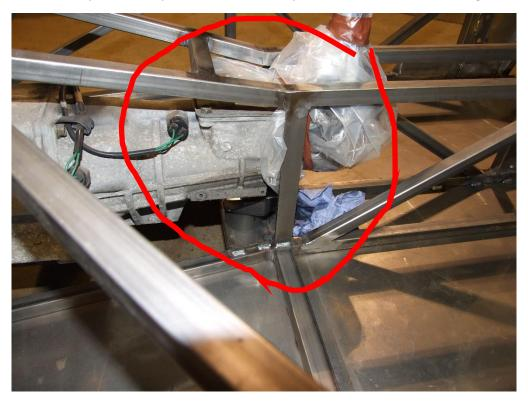
**TOP TIPS:** Ensure the starter motor is fitted when offering up engine to ensure it does not foul on engine bay diagonal. It's also worth checking that alternator, exhaust manifold and clutch master cylinder fit without obstruction.
