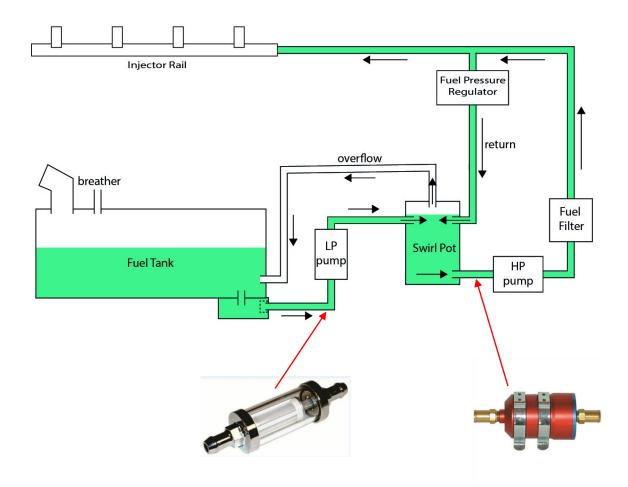
Option 2) In tank swirl pot. Swirl pot can be built into tank so that it feeds directly to high pressure pump and return enters direct from regulator. If designed correctly, slots in the front and back of pot enable fuel to enter the pot, but internal baffles and lack of slots to the sides slow down exit of fuel from pot when cornering. This should ensure there's always sufficient fuel in bottom of swirl pot, even at low fuel level in tank.
