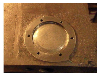
Plug fitted and 6BA holes tapped
