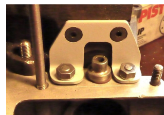
Front - straddles the cam bearing screw
