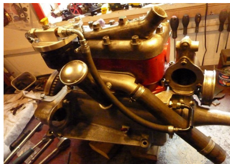
Full flow oil filter - return connection
