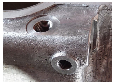
Return tapping on previous engine
