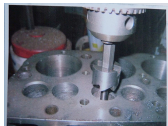
Boring for larger inlet valves
