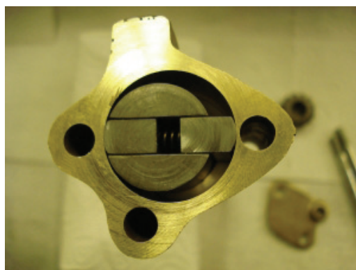
Heavily over-bored pump
