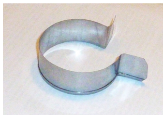
Improvised piston ring clamp
