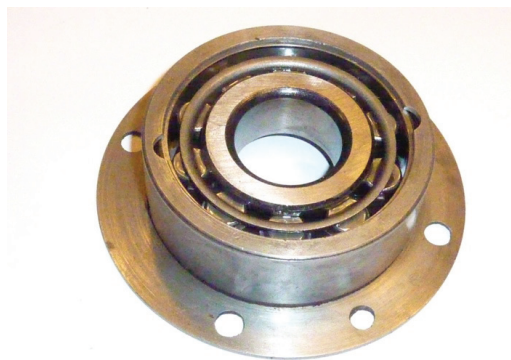
Rear main - showing housing cut-outs
