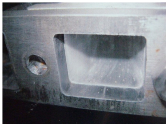
Smooth passage through manifolds
