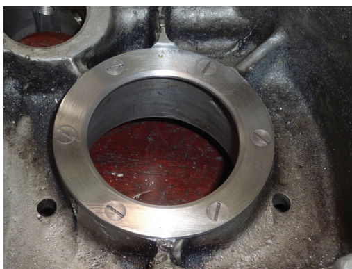
Replacement ring in position
