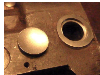
New core plug and clean seating
